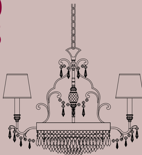
4010/S6+3 H 60 cm Ø 75 cm 6xE14x60w max 3xG9x40w max Paralumi / shade DAM-4010/16/IV
